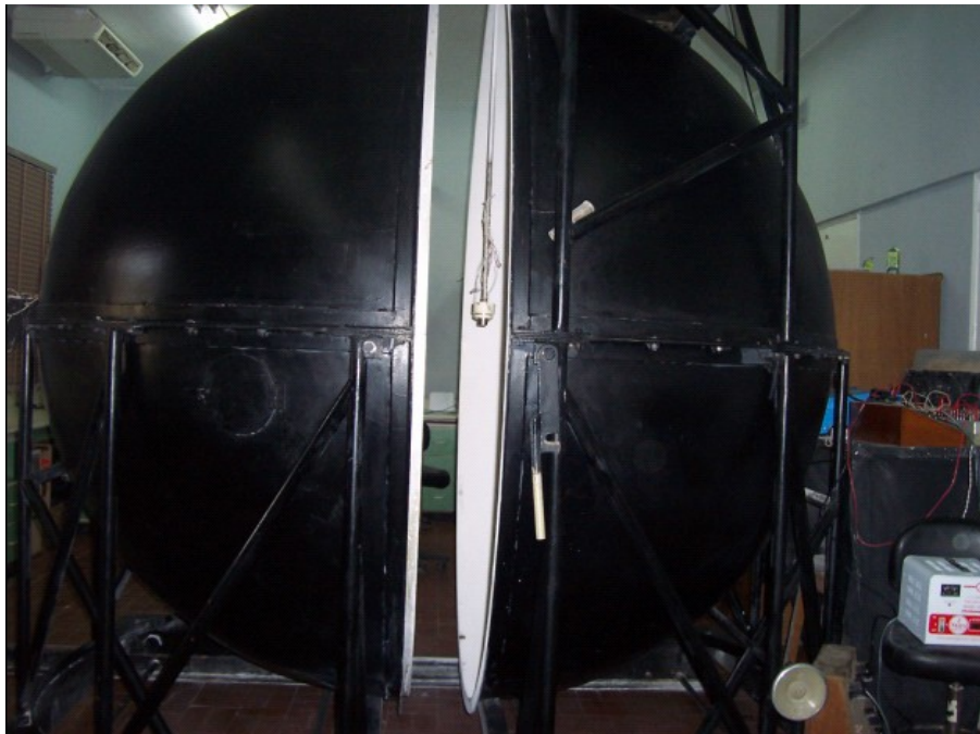
Figure.1 The NIS integrating sphere photometer system (2.5meter diameter)
